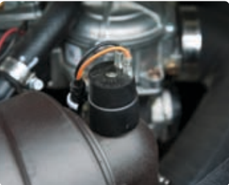
Electrically Monitored Air Filter Air cleaner sensor alerts the operator of a restricted air filter and allows replacement before damage.
