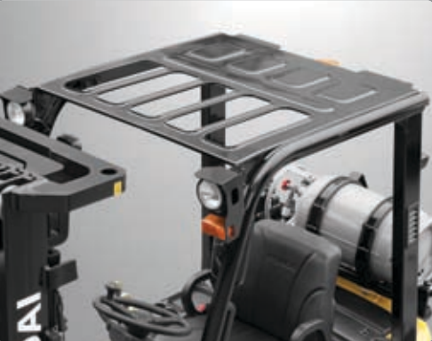
Strong Overhead Guard The safety overhead guard meets ISO 6055 regulation and protects the operator during hazardous jobs.
