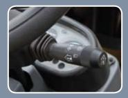
**Multi-function switch lever** Multi-functional switch lever gives easy access to lights and horn.
