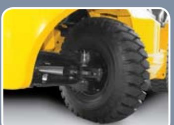
**Fully hydrostatic power steering**
