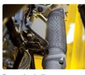
**Expansion bellows** The expansion bellows absorbs vibration and reduces noise generated from the exhaust gas system and also extends the life cycle of exhaust gas system.
