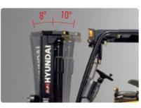
**Increased mast tilting angle** The mast tilting angle of 8 degrees forward and 10 degrees backward, the operator can safely and rapidly perform loading and unloading jobs.
