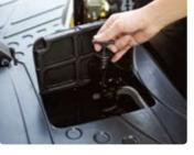
**Brake fluid reservoir** Highly visible, easily accessible reservoir **box for easy inspection** makes for quicker daily inspections.
