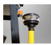
Visible precleaner Efficient, accessible pre-cleaner provides for longer engine life
