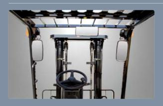
New high visibility for safe operation The operator is able to work with increased safety and accuracy due to a wider view mast.
