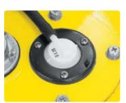
Fual tank safety valve Integrated safety check valve shuts off fuel supply in the unlikely condition of a truck overturn.
