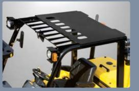
**Strong overhead guard** The safety overhead guard exceeds EEC and ANSI regulations and protects the operator during hazardous jobs.
