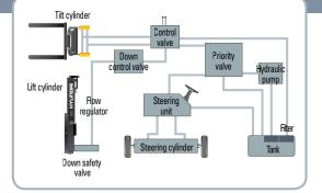
**State-of-the-art hydraulic system** The latest large-capacity hydraulic system reacts quickly during operation, and a low-noise control valve increases both efficiency and durability.
