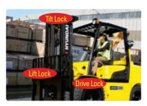
**OPSS (Operator Presence Sensing System)** Control of mast tilting, lifting and lowering is not possible through operation of the appropriate control when the operator is not in the seated position.(Option)
